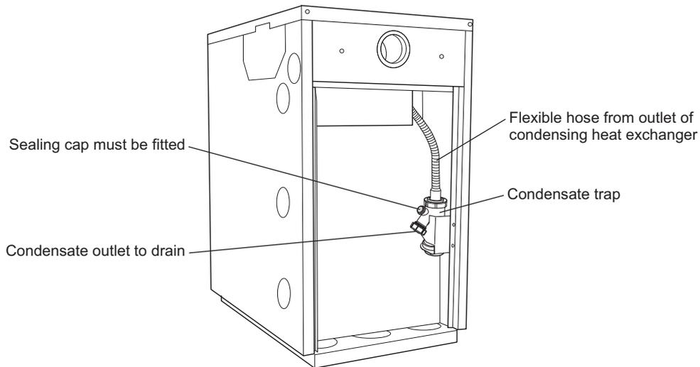
**Fig. 11 - All models rear view (panel removed)**
