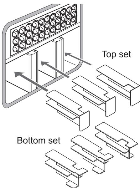
**Fig. 26 - 90/120 and 120/155 baffles**
