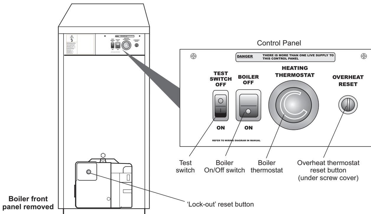
Controls for External modules - Fig. A
